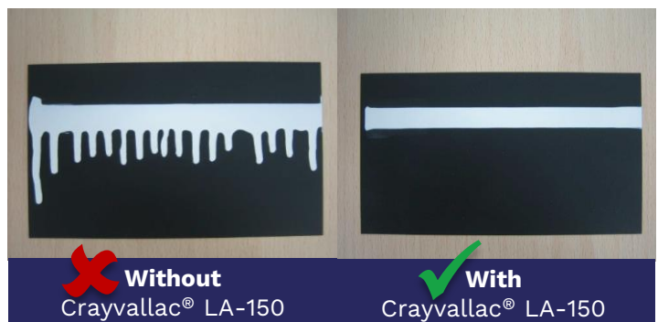
Application of a 200 µm wet thickness
